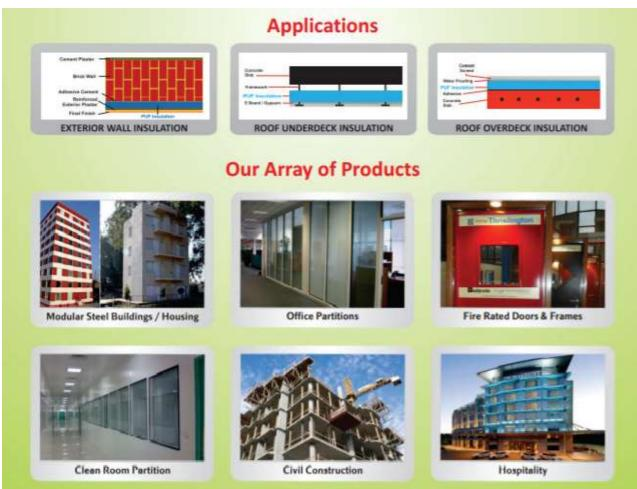
Synergy Prefab structures are made of Continuous Sandwich Panels (CSP) & manufactured off-site at our ISO 9001 : 2008 certified plant. Standard sections are easily assembled as per drawing & specifications. Panels options include Pre-Painted Galvanized Iron (PPGI) sheets, aluminium sheets, SS sheets or as directed.
